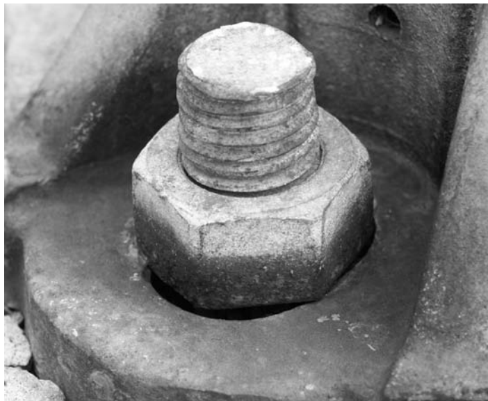
FIGURE 23.8. Galvanized bolting assembly after 10 years of exposure to deicing salt environment. (Courtesy of Kingston Technical Software.)
