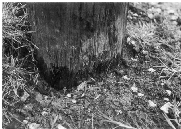
FIGURE 33.2. Soft rot on the surface of an 80-year-old creosoted utility pole below the soil surface.
