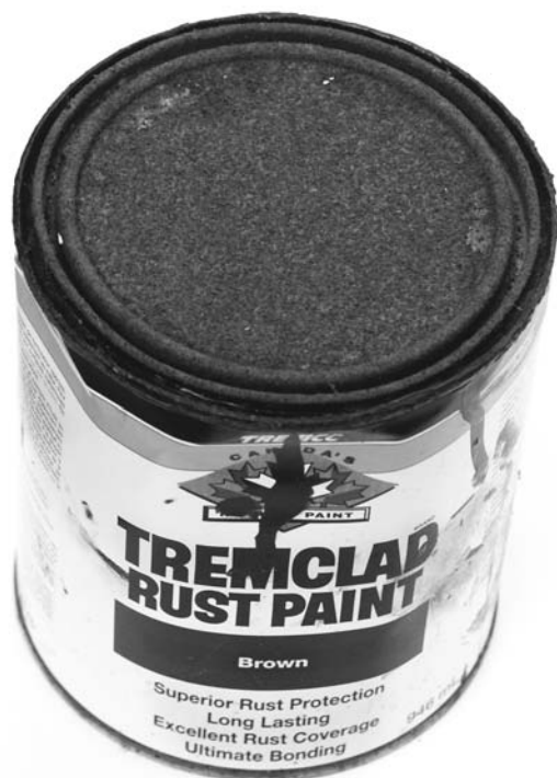
FIGURE 23.10. Rusted paint can after a few years in a normally humid basement. (Courtesy of Kingston Technical Software.)
