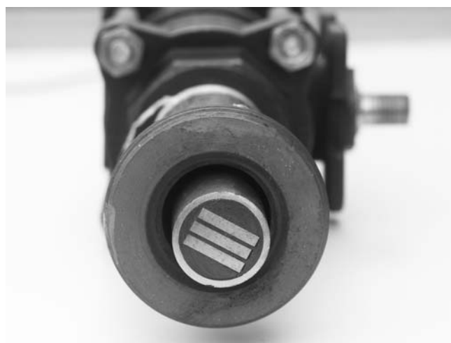
FIGURE 87.5. Close-up of corrosion sensing elements used for thin-film corrosion monitoring. (Courtesy of Kingston Technical Software.)
