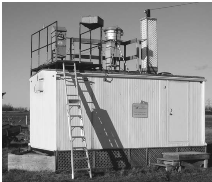
FIGURE 23.17. Deployable air quality monitoring unit on Montreal Island. (Courtesy of Kingston Technical Software.)
