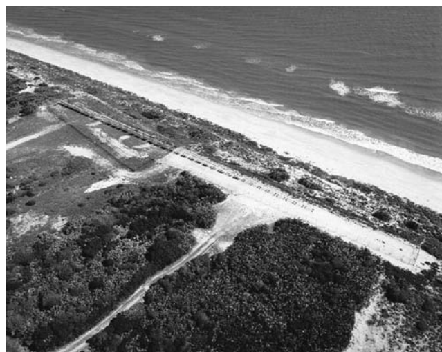
FIGURE 23.19. Aerial view of NASA Kennedy Space Center beach corrosion test site where atmospheric corrosivity is highest of any test site in continental United States.
