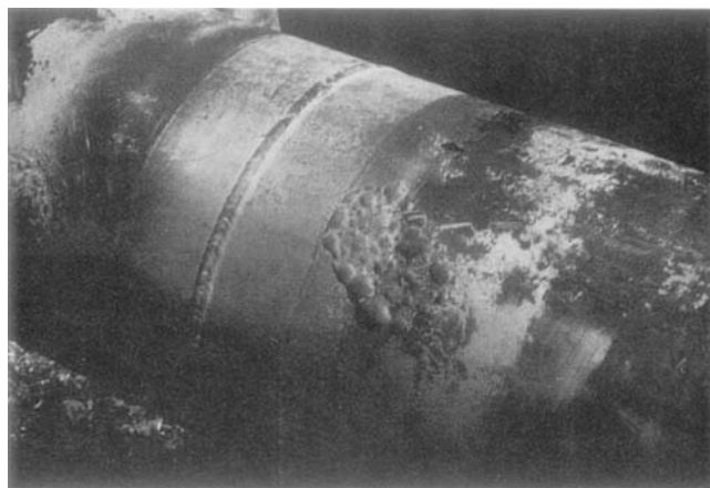
FIGURE 68.3. Blistering of FBE coating on hot pipeline ( 180^{\circ}\text{F} ). (Photo furnished by Lone Star Corrosion Services, Lancaster, TX.)
