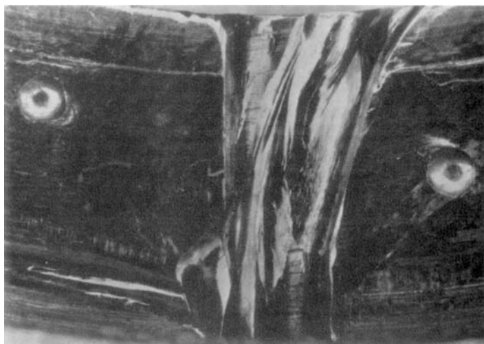
FIGURE 18.13. Wire drawing in a bronze cam ring for a hydraulic pump. (From Glaeser [51]. Reprinted, by permission of NACE International.)
