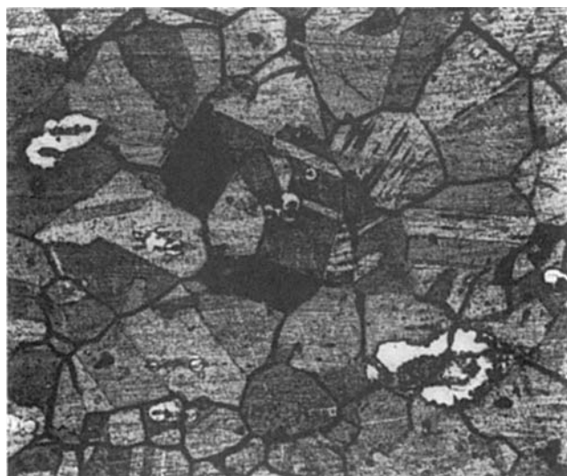
FIGURE 51.6. Initial attack in boiling 5% sulfuric acid on sensitized type 304 stainless steel [33] (250X). Steel: Heated 1 h at 675°C (1250°F). Exposure: 5 min. Structure: Intergranular attack, grains dislodged.
