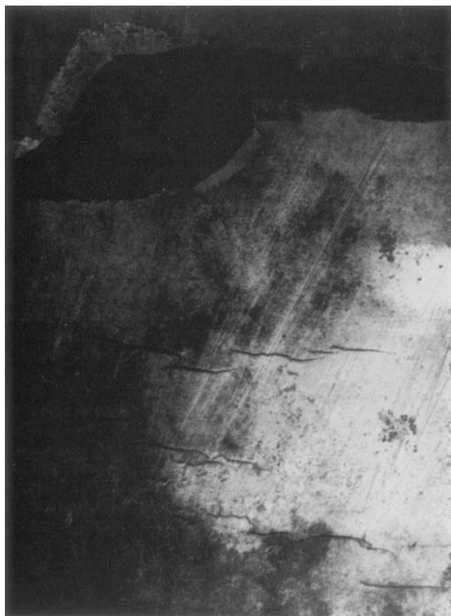
FIGURE 14.2. Secondary SCC on outer surface of high-pressure gas transmission pipeline near origin of SCC failure [3].
