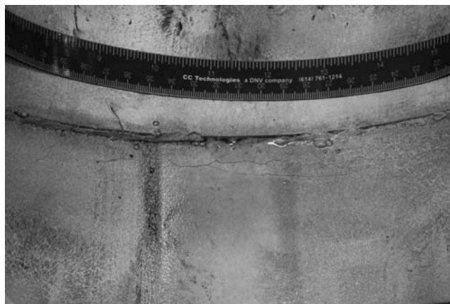
FIGURE 50.2. Photograph of the internal surface of API 5L Grade B piping used in ethanol service following magnetic particle inspection to reveal stress corrosion cracks.
