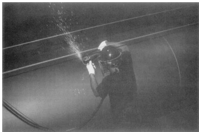
FIGURE 68.4. Inspection for and grinding of surface defects after blasting in FBE. (Photo furnished by EB Pipe Coating, Inc., Panama City, FL.)
