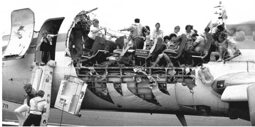
FIGURE 23.3. Boeing 737 operated by Aloha airlines after it lost major portion of upper fuselage in 1988.
