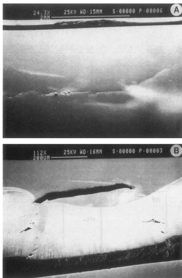
FIGURE 15.4. Two types of HIC. (a) centerline cracks and (b) blister cracks.
