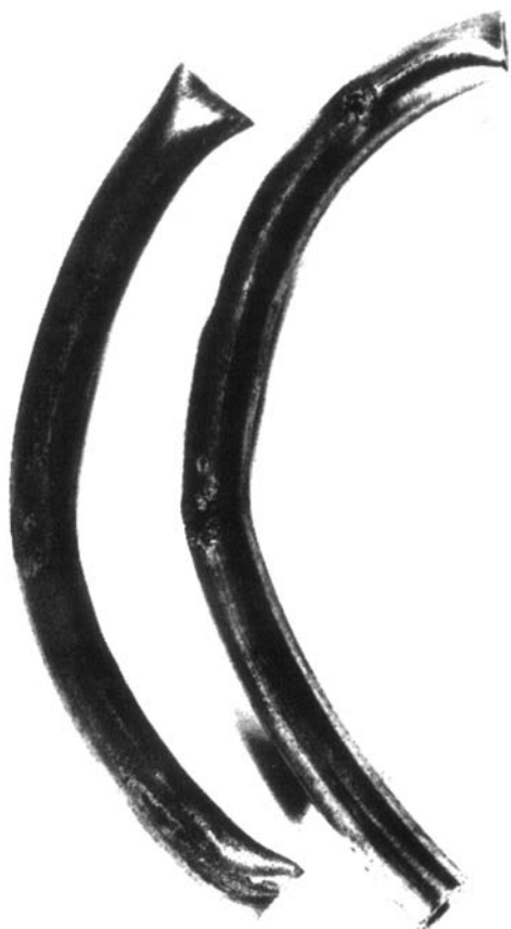
FIGURE 60.2. Allotropic modification and corrosion of tin; corrosion occurred in the specimen on the “outside” of the curve. (From [2]; reproduced by permission of iTRI.)
