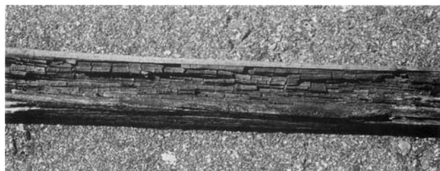
FIGURE 33.4. Brown rotted lumber showing typical darkening and cubical cracking.
