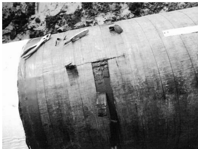
FIGURE 68.10. Mesh backed tape applied to pipe with condensation on one side. After three years in service, adhesion was very good on the dry side, but there was no adhesion on wet side, but the pH of the water under the coating was 11 with no corrosion on the pipe, proving the nonshielding properties of this coating system. (Photo provided by Polyguard Products, Inc., Ennis, TX.)
