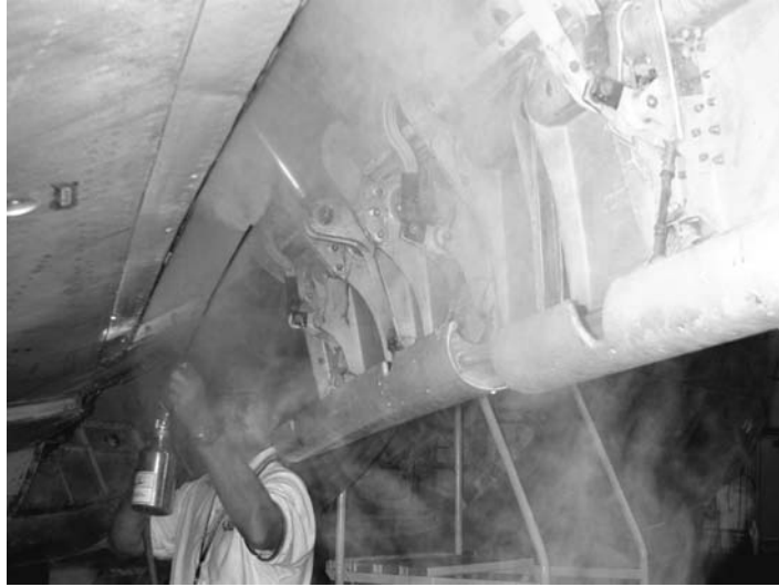
FIGURE 23.33. Fogging of aircraft with commercial CPC. (Courtesy Mike Dahlager Pacific Corrosion Control Corp.)
