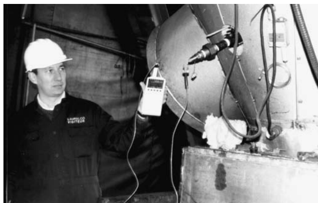
FIGURE 87.3. Field corrosion monitoring using electrochemical noise recorded with a hand-held data logger. (Courtesy of Kingston Technical Software.)
