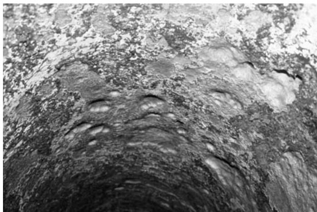
FIGURE 1.4. Severe corrosion of the inside of a stern tube. The pattern of general corrosion with some deeper pits is typical of low-carbon steel in seawater.
