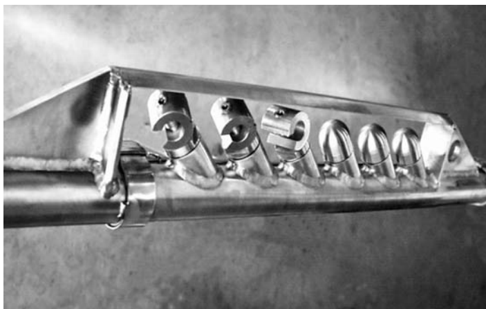
FIGURE 87.16. Detail of the Hanford site 25\text{-cm}^2 bullet and 47\text{-cm}^2 C-ring channel electrodes. (Courtesy of Glenn Hedgemon, HiLine Engineering & Fabrication.)
